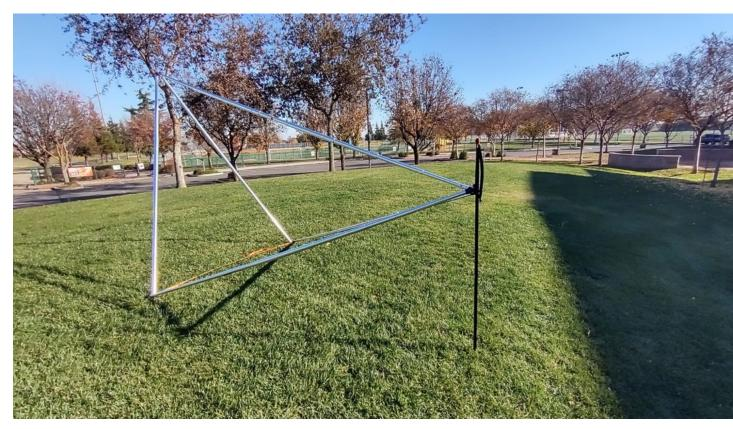
Set up on a significant head end down slope. One, this is the least recommended slope set up. Two, the head apex probably needs to be adjusted to the extreme upper position on the head support pole.
