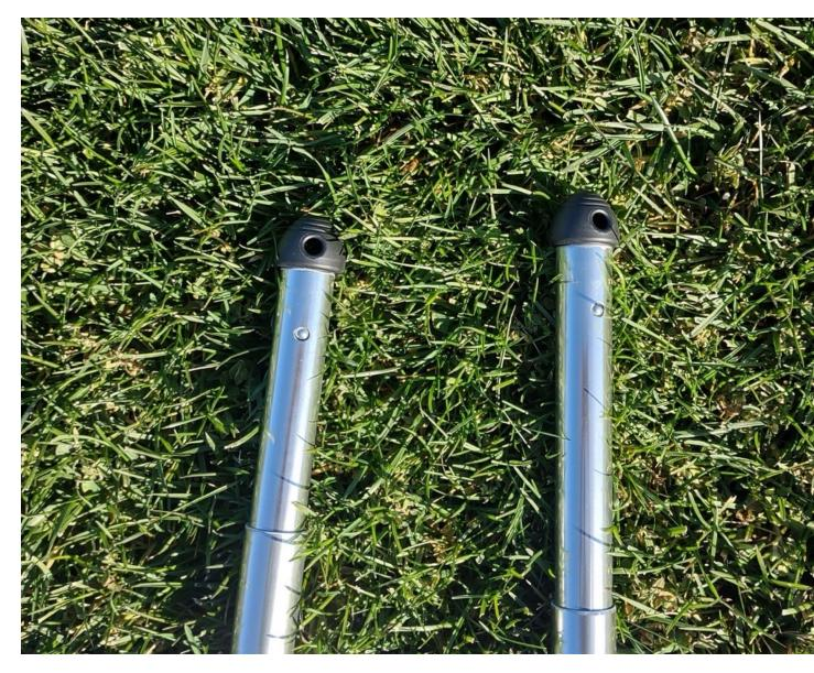
Take the orange baseline and set it at *approximately* 5 to 5-1/2 feet long. You can use your height as a guide. Lay this out on the ground so it makes a level line (cross slope). Take the 4-struts and extend them and place the feet next to the loops in the baseline as shown in the photo.
