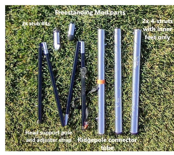
Now remove the #4 segments (one with the foot on it) from 2 of the 3struts and replace them with the stub #4s. These will go on the foot end of the stand. Set aside the full #4s you removed with the other unneeded Tensa4 parts.
