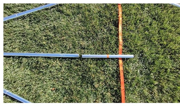
Now connect the ridgepole center connector (the one with the tape at the middle (which you can safely remove if you want) to one of the ridgepole 4-struts.
