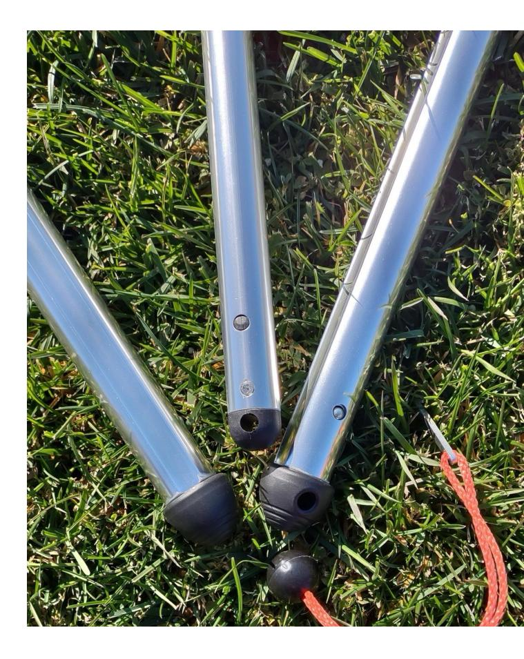
Using a ball-loop, thread the foot end as shown. Start by going through the end with no outer foot in the middle, then to one shortened 3-strut, and finally through the other shortened 3-strut. This order puts the ball toggle in the best location to suspend your hammock from it.
