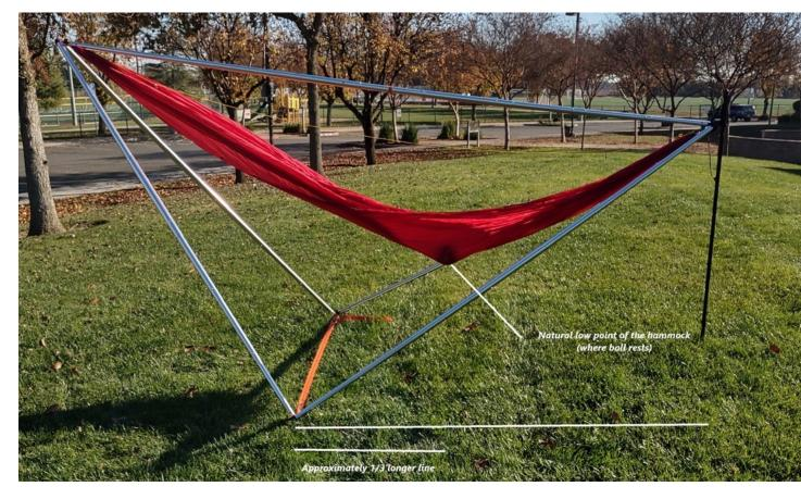
It is *CRITICAL* that the low point (where a ball rolls to and rests) of you hammock be on the head side of the baseline. YMMV, but about 1/3 of the way from the baseline to the Head Support Pole seems to be optimal. You can adjust the low point by raising or lowering the head apex, or by lengthening the hammock foot suspension, or both.
