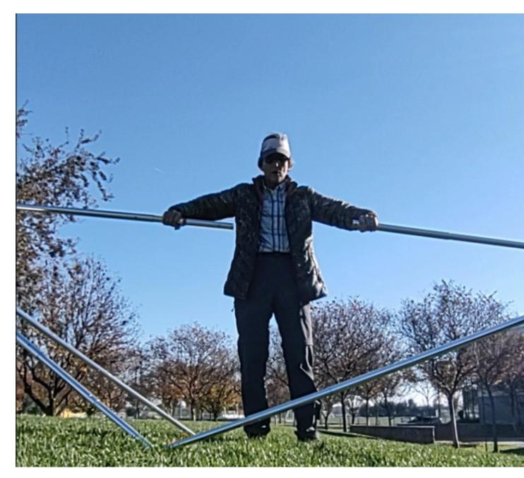
Grab both halves of the ridgepole and pull the stand upright and connect them together. I suggest standing on the side where you can see the spring button you are trying to engage. You can also use the Head Support Pole to 'pre-stand' up the head end of the assembly.
