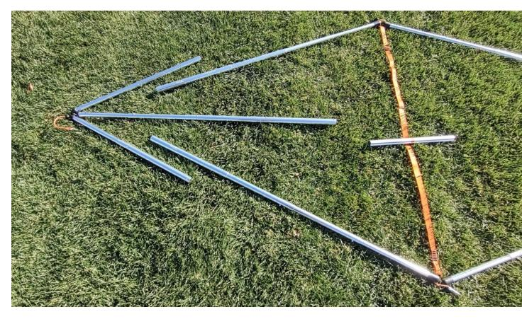
Now take the 2 shortend 3-struts and one of the FS-mod kit 4-struts (the ones without the outer feet) and extend them and lay them out as show. This is the foot end. Lay the center connection tube on the baseline.
