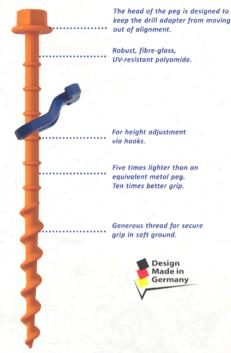
Soft, sandy grounds – Peggy (L)ong – PA with fibre-glass, with hook 31cm long, 17mm wrench size, torque max. 30Nm
