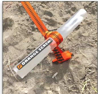
like a hook into the ground. First insert the stake through the holes in the end of the boom tube to make a figure 7. Point the boom toward the stand, and drive the stake in at an angle to keep the boom horizontal. Loop the end of the guyline over the end of the stake and under the tang, then twist the guyline around the boom end as shown right.
