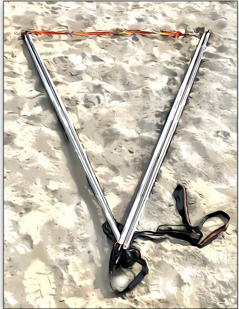
6. Attach the **black end** of a guyline to the bottom (foot end) apex, passing the pole connector line through one of the upper daisy-chain loops to leave a tail of loops inside the stand. These will be your hammock suspension. See step 10 for a peek at the end result.
