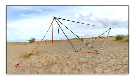
9. Attach and anchor the head end guyline. Its main purpose is to prevent the stand collapsing toward the foot side. Do **not** tighten it, now or ever. Leave it slack so the head end apex is free to move at least several inches. This allows both manual and dynamic adjustments, and avoids overloading the poles.
