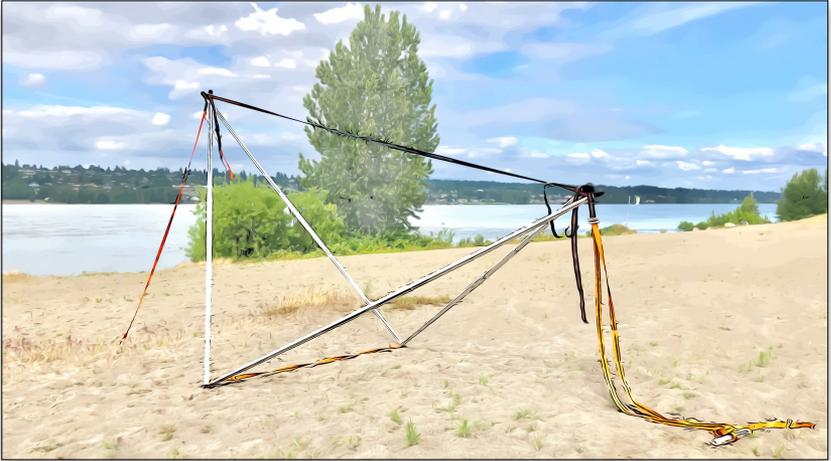
10. Hang the hammock. Those shorter than 12' (3.7M) need suspension to make up the difference with 12. So, a 10' hammock will need about 1' of suspension per side. With webbing, use carabiners in the daisy-chain loops of the guylines. With Amsteel, use your usual suspension method around one pole end per side, **not around both poles**. If your hammock has a ridgeline (cord between gathered ends), you may remove the stand's ridgeline to simplify adjustments.
