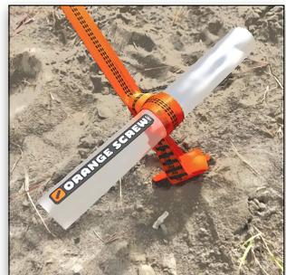
Point the boom toward the stand, and drive the stake in at an angle to keep the boom horizontal. Loop the end of the guyline over the end of the stake and under the tang, then twist the guyline around the boom end as shown right.
