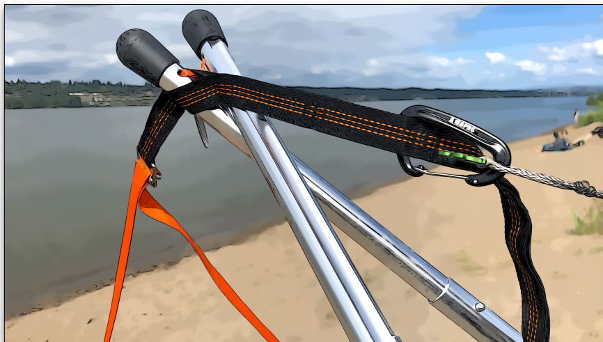
Detail of the finished state of the foot-end apex with webbing option, after the stand's ridgeline removed because hammock has its own.
