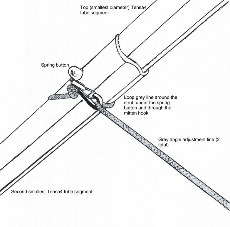
Tensa4 Tarp Extension - Strut connection detail
