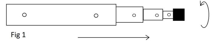
Connect the 4-section pole to the 3-section pole at the open ends. Repeat until you have 4 long poles. See Fig. 2
