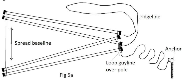
Unfold the stand and adjust the base position and/or guyline length so the tethered (foot) end is higher than the free (head) end. See Fig. 5C (no fig 5b)
