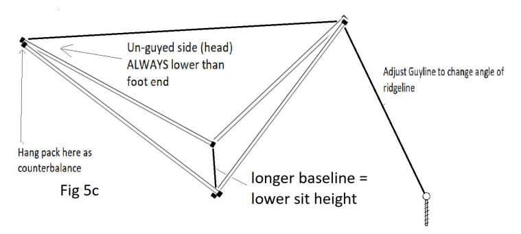
Loop the hammock suspension over one pole at each end and adjust the suspension and baseline length for your desired hang angle and sit height. See Fig 6
